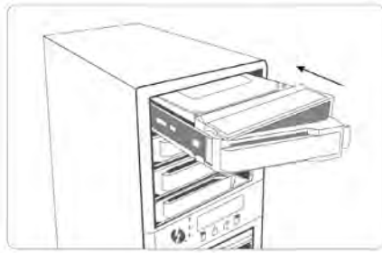
Figure 2-5, Sliding Drive Tray into Enclosure
