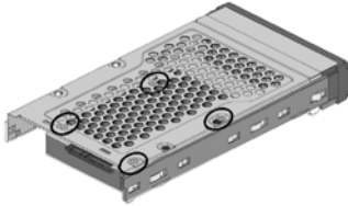
Figure 2-4-1, Installing 2.5-inch SATA Drive
