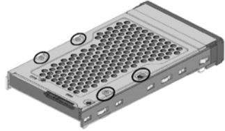
Figure 2-4-2, Installing 3.5-inch SATA Drive
