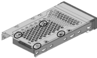
Figure 1-4-1. Installing 2.5-inch SAS/SATA Drive
