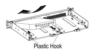
(3) The Mac mini must be inside the anti-vibration posts.
