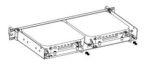
(6) Install the top cover by fitting the cover and attaching the three (3) screws.
