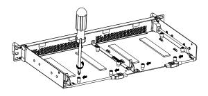
(2) Incline the Mac mini and push back the plastic hook. Insert the Mac mini so the plastic hook is positioned to the on/off button.
