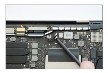
Slide the pointed end of a spudger underneath each antenna cable close to the connector and carefully use a levering motion to release each connector.
