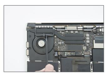
The audio cable is adhered to the fan using light adhesive. Carefully peel the cable away from the fan to about halfway. Do not fully remove the cable from the fan.
