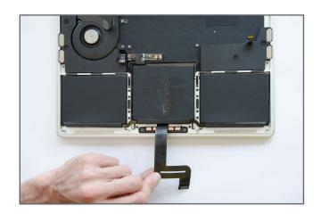
Carefully open the Macbook while keeping the display flat and guiding the trackpad cable around the battery. Once the cable is clear remove the trackpad.
