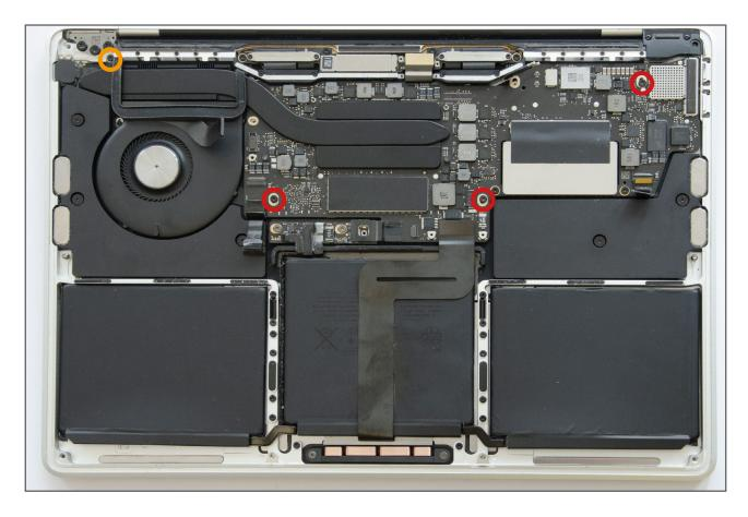
Using a Torx T5 screwdriver remove one small screw from the end of the heatsink and 3 larger screws from the logic board as depicted in the image. These screws will need to be returned to their original positions when reassembling.
