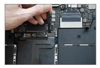
Using the flat end of a spudger lever the trackpad cable directly up from the logic board.
