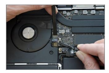
Using the flat end of a spudger carefully lift the locking lever on the speaker cable connector.
