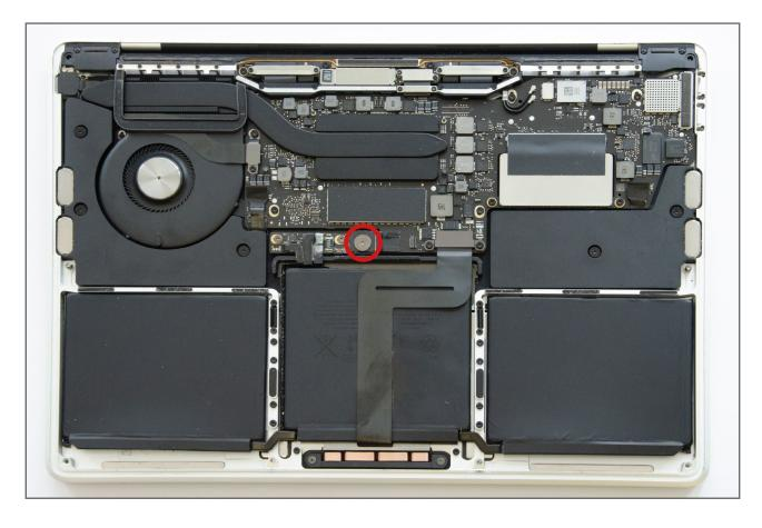
Using a Torx T5 screwdriver remove the large flat screw from the main battery power connector.
