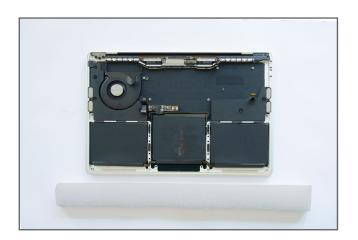
Place the MacBook on a book or foam wedge so that the laptop tilts backwards. This will help the solvent flow underneath the cells and penetrate the adhesive.
