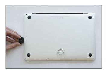
Move the pick around the edge and up to the middle of the left side. You should hear and feel a pop as the first securing clip is released.
