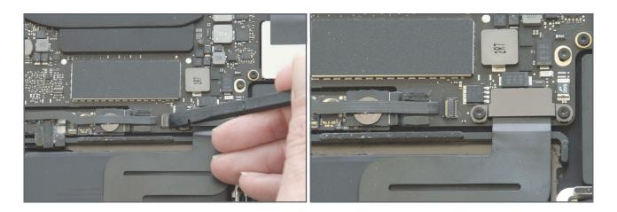
Using the flat end of a spudger carefully lift the locking lever on the battery cable connector.
