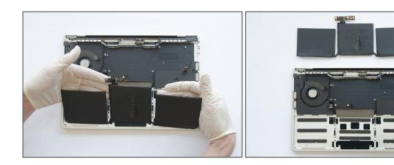
Once the middle cell is fully released the battery can be lifted out and removed.
