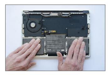
When you are satisfied that everything is correctly fitted and aligned apply light pressure to each of the cells to fully activate the adhesive.
