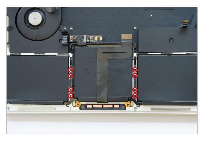
Using a Torx T5 screwdriver remove 8 larger screws and 2 smaller screws as depicted. These screws must be returned to their original position when reassembling to prevent damage to the trackpad
