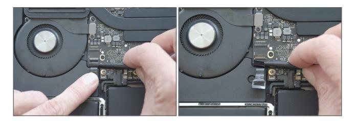
Carefully slide the keyboard cable out of the connector. It may help to slide the pointed end of a spudger under the cable and use this to carefully slide the cable out.
