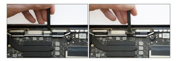
Using the flat end of a spudger carefully lever the display cable directly up from the display board.
