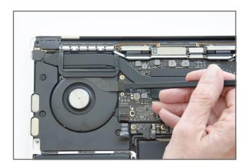
Using the flat end of a spudger carefully lever the audio board cable directly up from the logic board.
