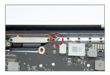
Special attention should be paid to the antenna cables as you may need to hold the cables out of the way while you maneuver the logic board around them.
