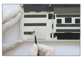
This can involve a lot of work, so be patient. Using more solvent on the adhesive patches can help with the removal of them.
