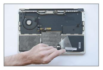
Carefully peel off the plastic cover on the top side of the battery.
