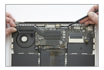
Carefully lift the logic board from the left while checking for snagged cables. If you feel resistance stop and review the previous steps to ensure that all cables have been correctly disconnected and that all logic board screws have been removed.
