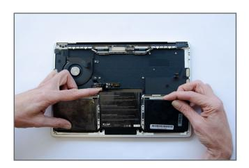
Carefully place the battery into the housing while paying particular attention to the alignment of the battery board screw holes.
