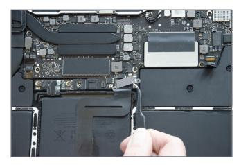
Remove the securing bracket.
