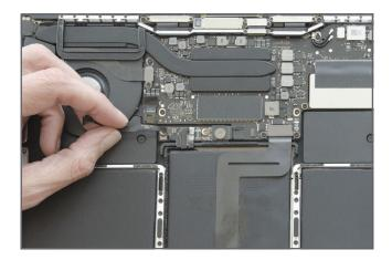
Using pointed end of a spudger to lift the locking lever of the small connector at the other end of the battery cable.
