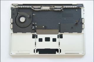
Finally wipe the entire area with an isopropyl wipe to ensure that the adhesive of the new battery adheres correctly. Allow the area to dry before attempting to install the new battery.
