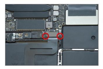
Using a Torx T5 screwdriver remove the 2 screws holding the track pad cable securing bracket.
