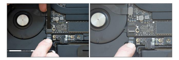
Using the flat end of a spudger carefully lift the locking lever on the keyboard cable connector.
