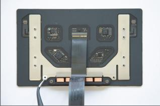
The trackpad has 6 metal shims around the screw holes. Be careful not to lose these as they come away easily. If a shim does come away use tweezers to place the shim back on the trackpad.
