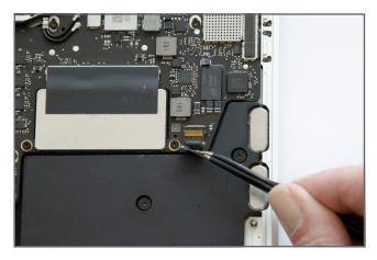
Slide the speaker cable out of the connector.
