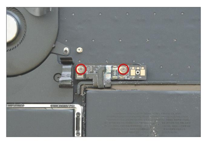
Using a Torx T5 screwdriver remove 2 screws from the battery board.
