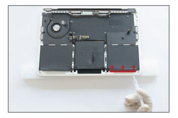
You do not need to use a lot of solvent. The supplied bottle is more than sufficient to remove all of the cells.
