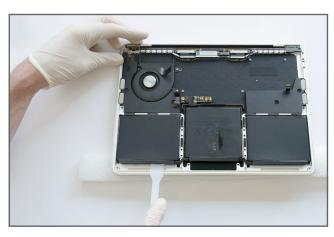
After around 2 minutes insert the sharp end of the spatula underneath the left cell. It's best to orientate the spatula so that the flat side of the sharp end is upwards - see image.
