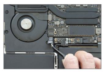
Slide the speaker cable out of the connector and move upwards to reveal the keyboard cable and connector.
