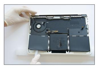
Work the spatula under the cell. Use a wiggling motion along the entire length of the cell to release the adhesive.
