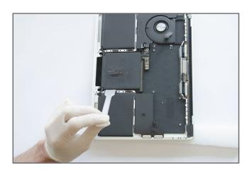
Carefully use the sharp end of the spatula, this time with the flat side down. Work along the right side carefully levering the cell up to loosen the adhesive. Be patient and keep levering the cell bit by bit until the adhesive releases enough to be able to fully insert the spatula. Then work with a wiggling motion to release the remainder of the adhesive.
