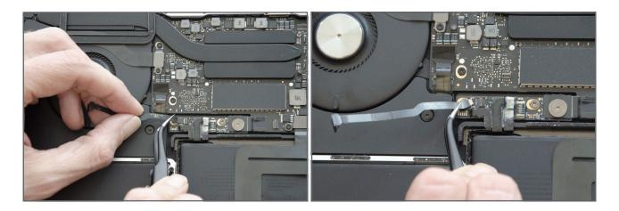
Slide the battery cable out of the connecter and store it. The cable will be required for the new battery.
